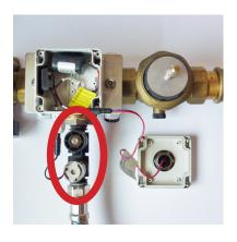
Clean the electric valve; Install fine filter (K&K Art. No. 3990039); or clean existing filter
