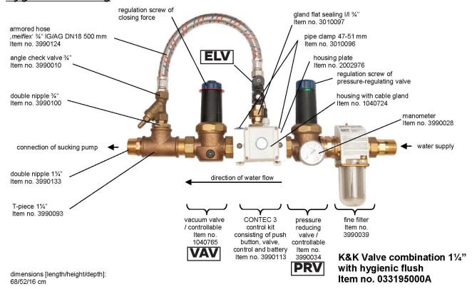
After the fine filter, a pressure reducing valve (**PRV**) is arranged first in the direction of flow, which serves to reduce the water of a supply line, which is present at an undefined pressure (but at least 3.0 bar), to a constant pressure of 3.0 bar, which is necessary for the correct functioning of the system.
