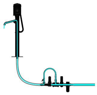
The hygiene flush is set to a 12-hour rhythm and 30 s runtime in the factory. This will flush 6m of DN 40 pipe.
