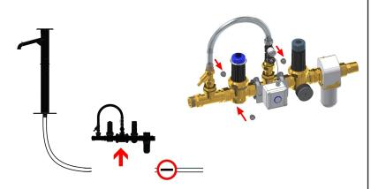
Replace the piercing valve in the sealing seat.
