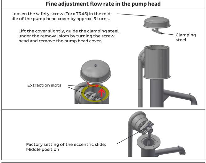
Loosen the 4 clamping nuts (M8 – spanner size 13 mm) on the eccentric slide by 1-2 turns.
