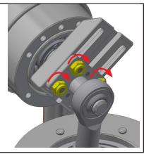
Place the pump head cover and clamping steel on the pump head and screw tightly again with the safety screw.
