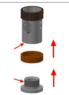
7. When assembling the pump piston with the connecting rod and the axle, the installation directions of the spacer sleeves in the pump piston (radius in the direction of the piston skirt) and the orientation of the outlet bore must be observed.
