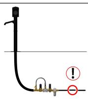
Unscrew the black plugs on the K&K valve combination (= 3 pieces in total).
