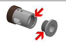
6. Before assembling the piston parts with the new leather sleeve, the threads must be provided with a thread locking adhesive (Loctite or similar), in order to prevent unintentional loosening during operation.
