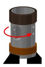
4. Insert a suitable tube or round material as a lever into the oval outlet hole of the upper piston section. By turning the upper part of the piston anticlockwise (right-hand thread), the upper part of the piston and the lower part are released from each other.
