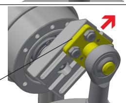
Small displacement = small flow rate = small pumping resistance
