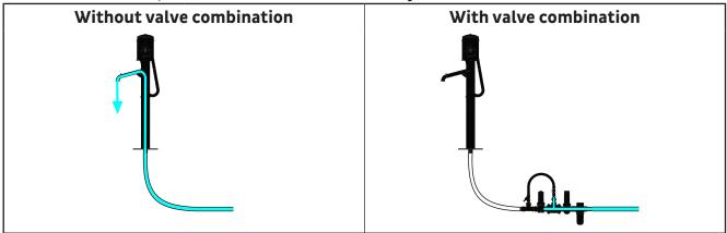
If negative pressure is generated at the outlet side of the valve combination, the valve combination opens the flow and releases until atmospheric pressure is again present at the outlet side:
