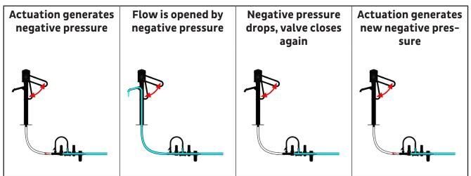
If the K&K water pump and K&K valve combination are connected correctly in accordance with the K&K installation instructions and the specified maximum distances are observed,
